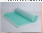
PA-99 made of glass fiber fleece and is used effectively to arrest the paint mist in spray booth.PA-99 Pads are designed to collect most of Paint overspray. Maintenance problem and hazards of fire are reduced due to non accumulation of paint layer. Cleaner air is discharged to atmosphere as well.
